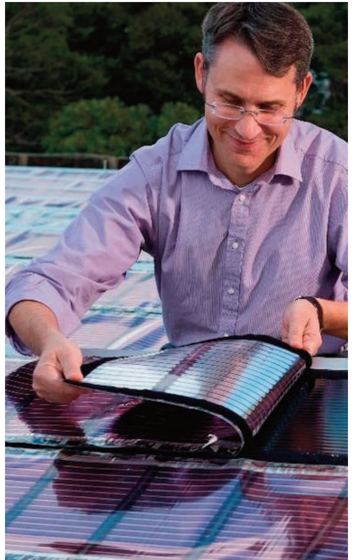
Printed solar creator, University Of Newcastle's Professor Paul Dastoor, unveils their first solar demonstration on a factory roof in Newcastle
